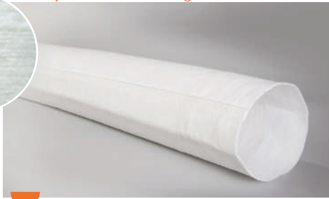
Polyester Keçe Filtre Torbası ( kenar dikişli ) ( 250 lt/dm 2 /min - Ø 12,5 cm / 180 - 300 cm ) Polyester Needle Felt Filter Bag ( with seam )
